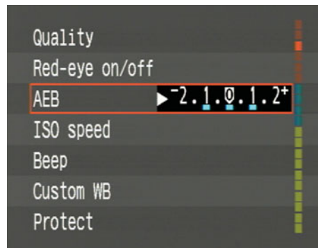
FIGURE 8.23 If your camera has an autobracketing feature, you can set it to automatically shoot a series of bracketed exposures.
